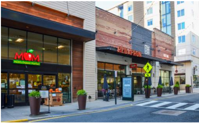
(Left). Freestanding retail frontage uses varying parapet heights to screen mechanical and utility equipment on the roof. (Right) Retail village with farm-style shed roofs with clerestory roof projections create voids within roof forms to discretely hide mechanical and utility equipment
