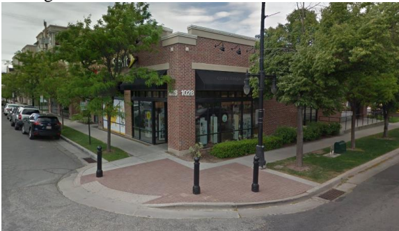
Figure 10. Bulb-out provides traffic calming and shorter pedestrian street crossing distances.
