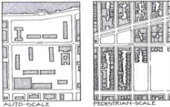
Figure 7. Pedestrian scale street layouts include shorter blocks and a greater level of connectivity.
