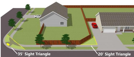
Figure 1. The 6-foot side yard fencing does not extend into the required 35-foot or 20-foot sight triangles. The fencing must be constructed diagonally along the edge of the 20-foot sight triangle to maintain clearance.
