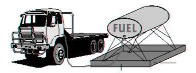
SLOPED OR OTHERWISE DESIGNED FOR EASY REMOVAL OF LEAKED FUEL
