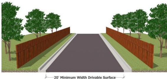
Figure 5. Typical 20-foot flag lot driveway cross section includes a 20-foot wide drivable surface and appropriate
