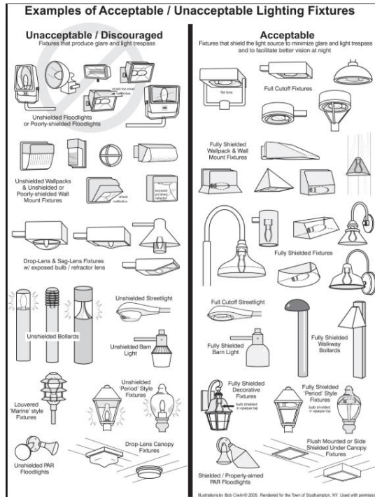
Figure 8 illustrates the acceptable and unacceptable lighting fixtures.
