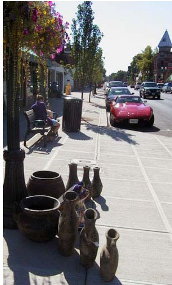
Bulbouts at intersections provide pedestrian "breathing room" and opportunities for seating, enhanced landscaping and other embellishments
