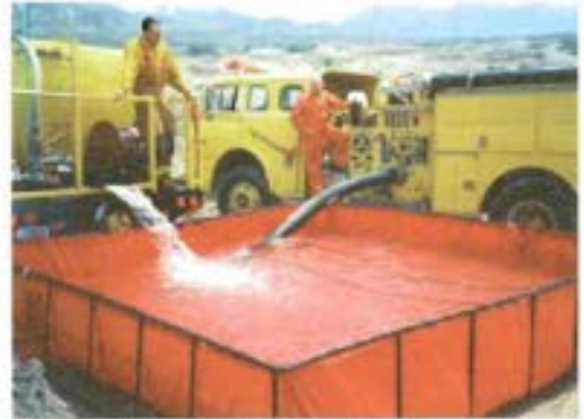
Figure 105 Drafting out of a drop tank
