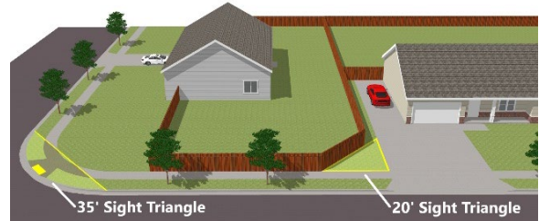
Figure 1. The 6-foot side yard fencing does not extend into the required 35-foot or 20-foot sight triangles. The fencing must be constructed diagonally along the edge of the 20-foot sight triangle to maintain clearance.
