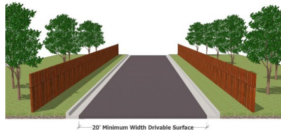
Figure 5. Typical 20-foot flag lot driveway cross section includes a 20-foot wide drivable surface and appropriate drainage improvements.
