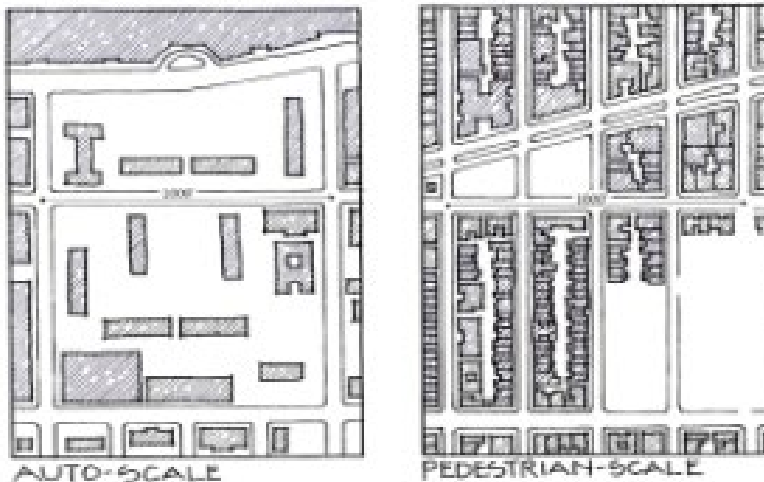
Figure 8. Pedestrian scale street layouts include shorter blocks and a greater level of connectivity.
